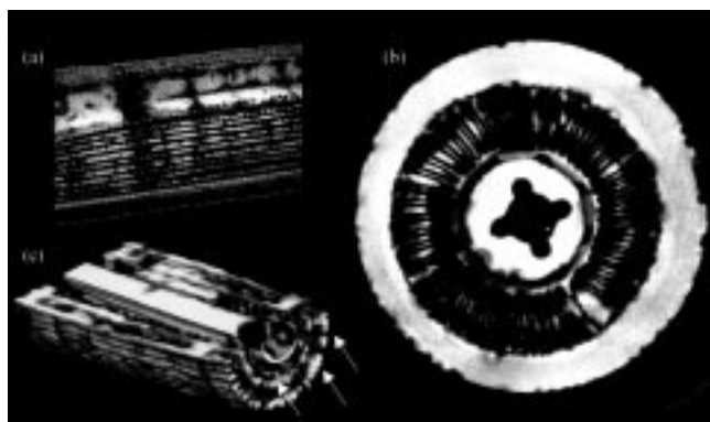
Figure 4. (a) Section of a partially blocked filter showing banding of contaminant deposition; (b) 2-D image of a 5-mm transverse slice through the same blocked filter in the housing; (c) 3-D rendered MR image of a 12-cm section of the same blocked filter.
